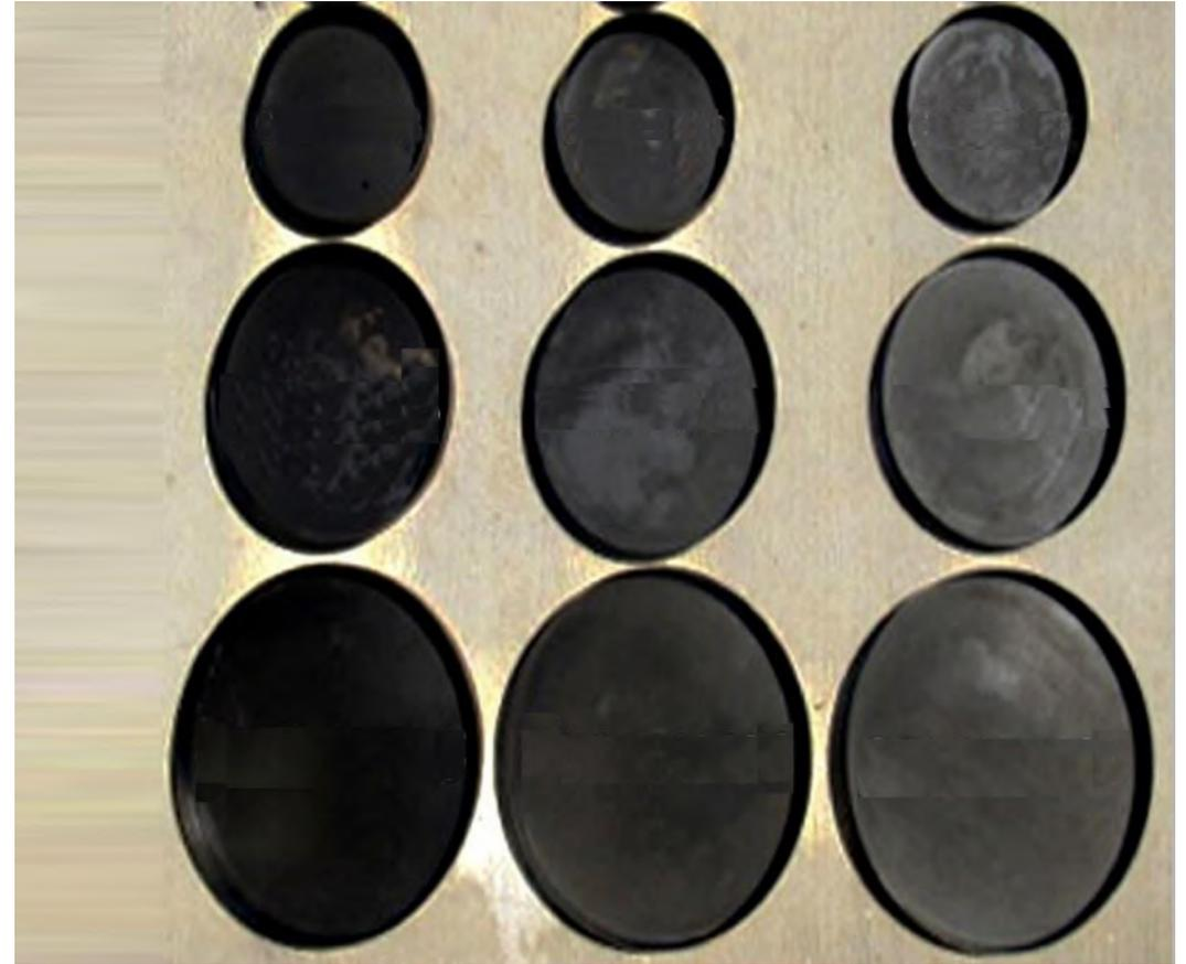
Pans of 200 mm dia, 40 mm depth made of Stainless Steel (SS), Mild steel (MS), Aluminum alloy (Al) and glass (GL) (clockwise from the top) on left side and pans of 300, 400 and 500 mm diameter, 40, 50 and 60 mm depth made of MS on the right side
