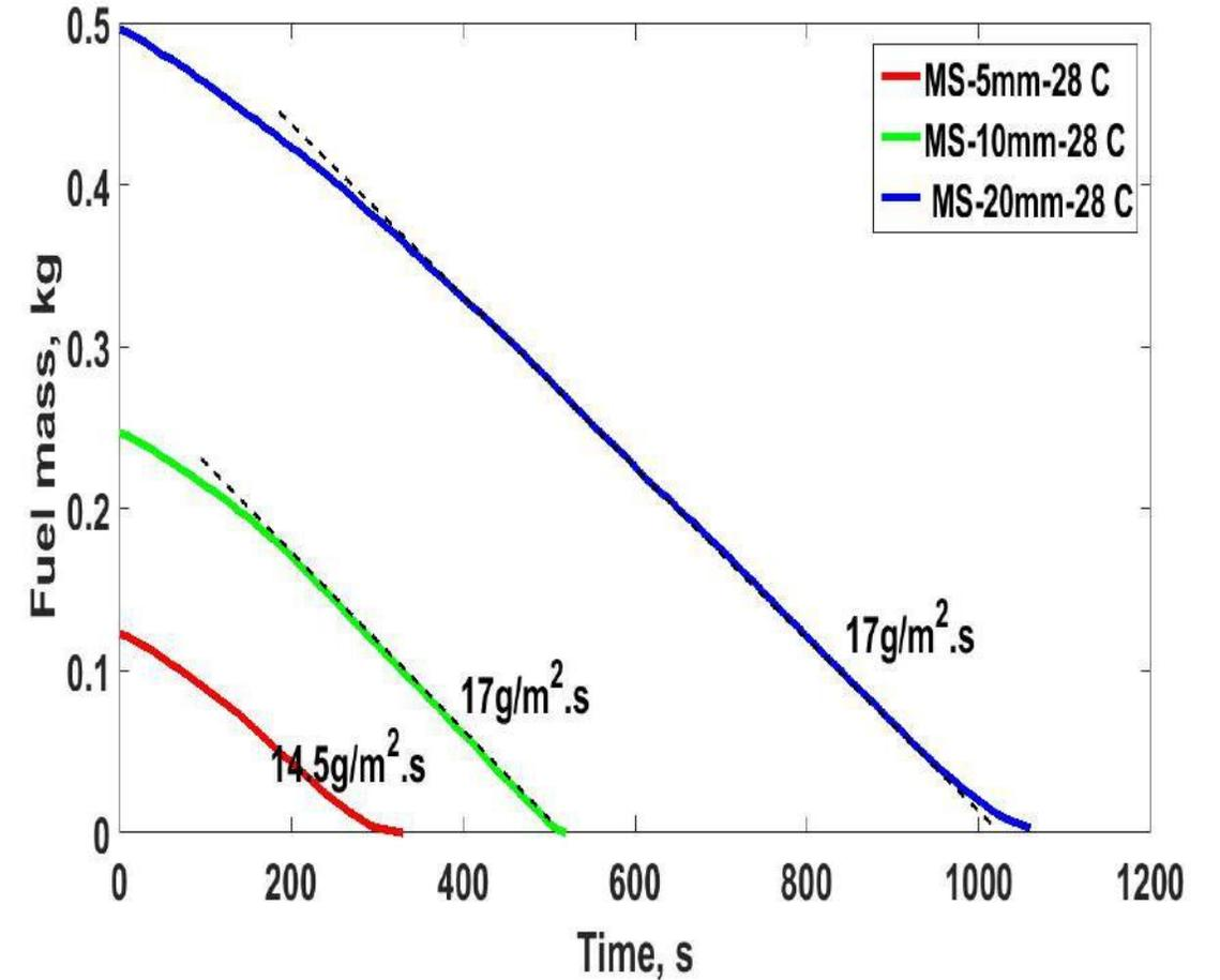
Fuel depth effect on burn rate is negligible for methanol and ethanol
