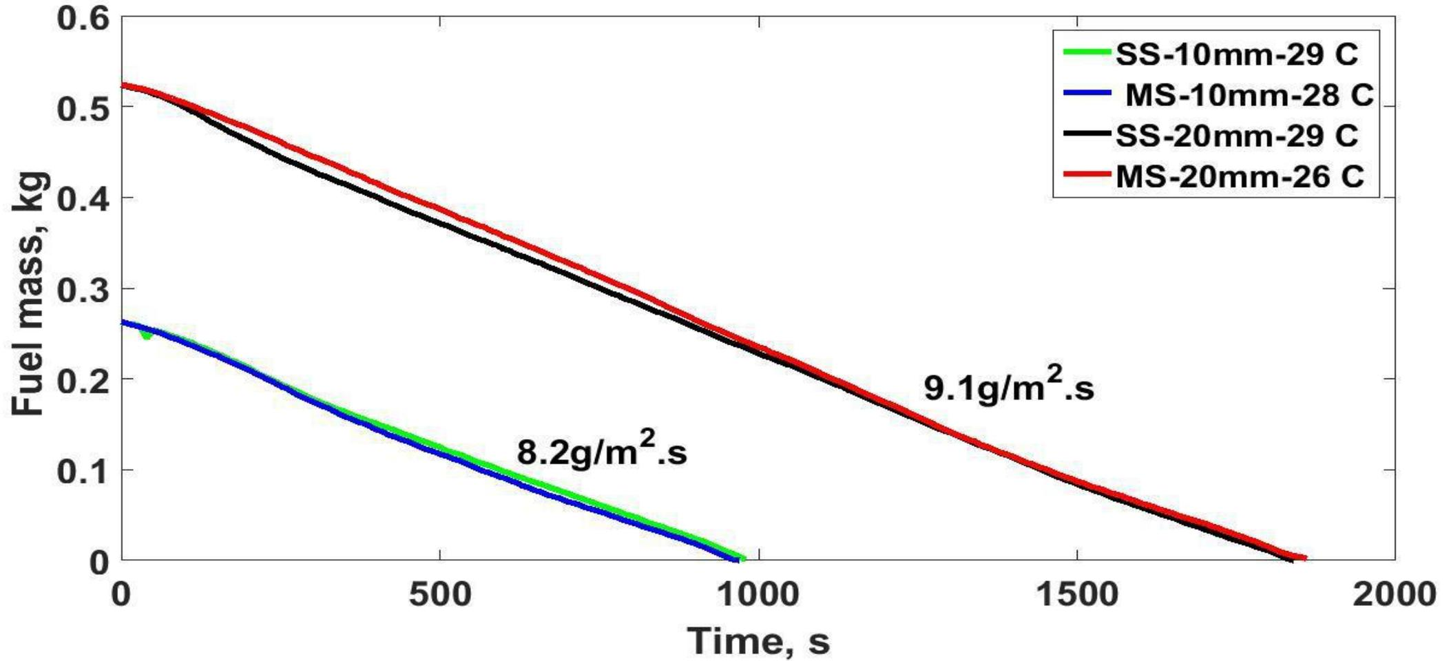
Fuel thickness and material effect on the burn rate is negligible for diesel fuel
