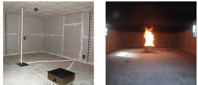
Figure 6. Photograph of test area and flame ~33 s into the test: A-Pan; B-Vertical scale; C- Thermocouple tree; D- Coated Roof
